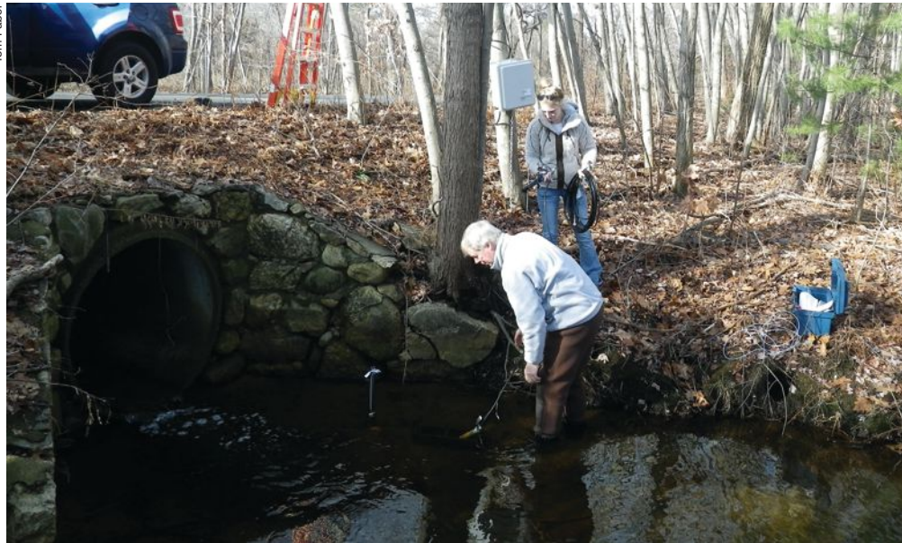
Near-real-time testing of temperature and conductivity of highway runoff
